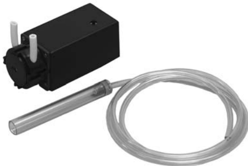
LM3-WXM Water eXchange Module – LiterMeter III Pump mounted in plastic box with built- in Liquid Level Control (LLC). Interrupts power to pump when high liquid level is reached. Connects to LiterMeter III for power and control. 5.4" x 2.2" x 2.2" (13.7 cm x 5.6 cm x 5.6 cm)
