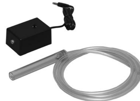
LM3-TCM Top-off Control Module – Plastic box with built-in Liquid Level Control (LLC). Connects to 12V input of LiterMeter III to interrupt power when high liquid level is reached. 3.0" x 2.0" x 1.7" (7.6 cm x 5.1 cm x 4.3 cm)
